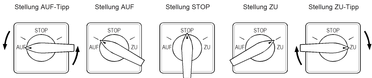
Figure 3: control switch S31
